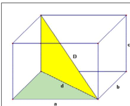
$$\begin{aligned} D^2 &= c^2 + d^2 \\ d^2 &= a^2 + b^2 \\ D^2 &= a^2 + b^2 + c^2 \end{aligned}$$
